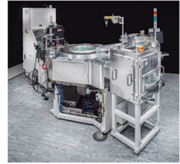
Mosaic™ system for plasma dicing of framed 300mm wafers
